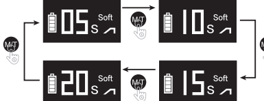
Schematic diagram of curing time setting interface
