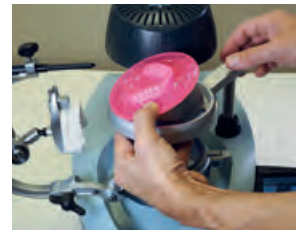
10. Release foil securing ring, remove the Occluform model pot with the foil.
