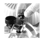
1. When the closing power of the arresting joint gets weak, add oil. Therefore completely open the black nut and pull it out.
