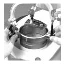
1. Put the Occluform-3 with the fixation ring onto the 3d-housing at right angles to the unit (supporting pin to the right).
